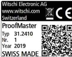
The rating plate of the ProofMaster is located on the reverse of the device and contains the following information:
