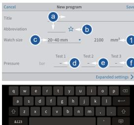
The screenshot shows the 'New program' dialog box. It has fields for 'Title', 'Abbreviation', 'Watch size', and 'Pressure'. There are three test slots: 'Test 1', 'Test 2', and 'Test 3'. A keyboard is visible at the bottom of the screen.
